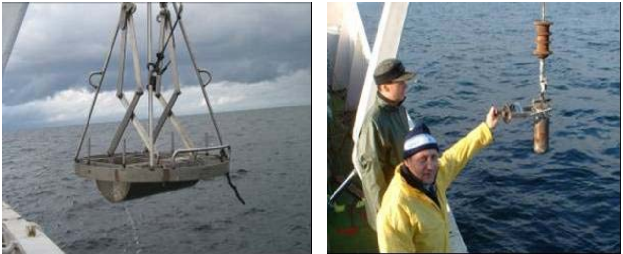
Fig. 4.2 – Sampling procedure. Taking up sediment samples using the Wan-Win and the DTSh-3 small corer
